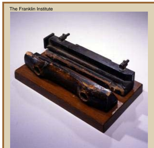
Slug mold (~10 in.), into which hot lead is poured to create "slugs" of metal from which individual characters (letters, numerals, etc.) can be made
