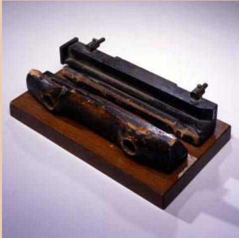
Slug mold (~10 in.), into which hot lead is poured to create "slugs" of metal from which individual characters (letters, numerals, etc.) can be made
